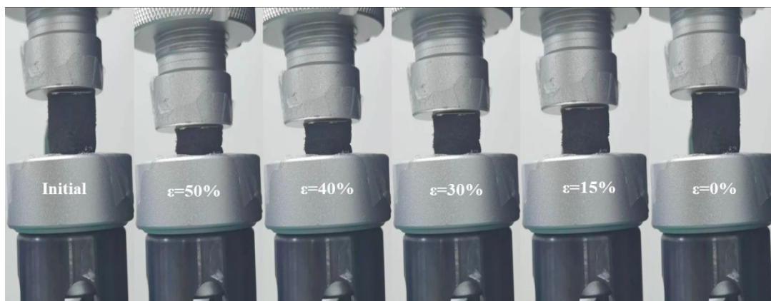
Figure S22. Digital photo of the instantaneous compression process of the PIF/CNTs composite aerogel at a speed of 500 mm/min.
