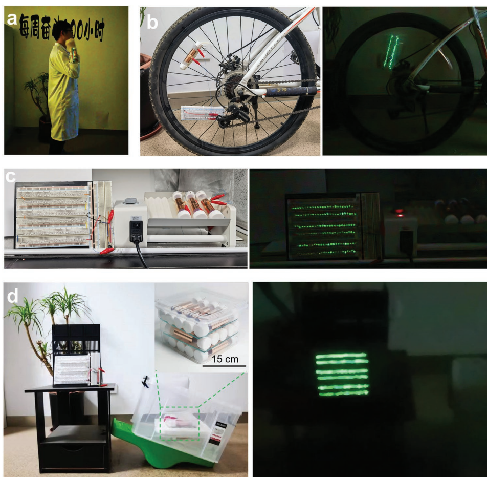
Figure 4. The application of the STVE-TENGs. a) 24 LEDs are powered by a STVE-TENG as wearable energy supply devices. b) Demonstration of the STVE-TENG for harvesting the mechanical energy of rotating bicycle wheels. c) Demonstration of lighting 150 LEDs through 3 working STVE-TENGs. d) The power package composed of 15 STVE-TENG was used to recover wave energy and lit 150 LEDs.
